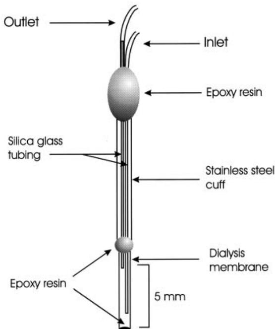
**Figure 4.6** The tip of a microdialysis probe, expanded to show dialysis tubing around a steel cannula through the base of which fluid can flow out and then up and over the membrane. The length of membrane below the probe support can be altered (1–10 mm) to suit the size of the animal and the brain area being studied. Flow rates are normally below  $2 \mu\text{l}/\text{min}$
